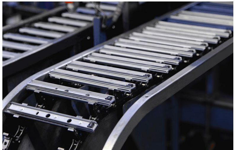
In-house developed Schock assembly line for production of linear slides.
